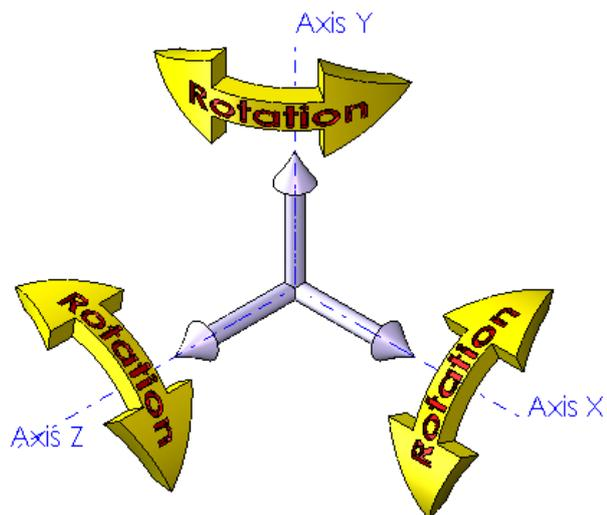
Once all the six degrees of freedom are fixed, the position and orientation of an object is considered 'fully defined'.
