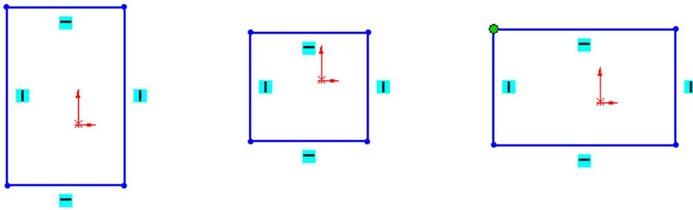
**Under-defined conditions** allow designers to drag and change the shapes on screen freely. The object remains a rectangle no matter how it is changed because it is only governed by the geometry relations.
