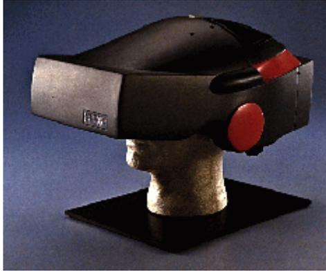
An HMD (Head-Mounted Display) is a headset with two small monitors installed inside, each for an eye to present a stereo view of the virtual world.
