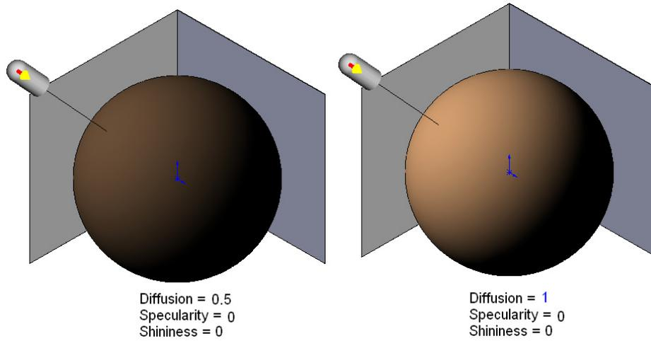
Specular reflection is the opposite of diffuse reflection. An ideal specular reflection reflects a ray into a single outgoing direction without any scattering. For example, mirror is an ideal specular reflection.
