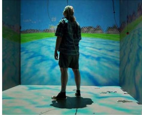
CAVE (Cave Automatic Virtual Environment) is a system for projecting images on the wall, floor and ceiling in a chamber.
