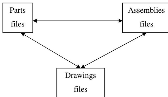
The three dimensional data of parts and assemblies on shapes, dimensions, etc can be projected onto 2D drawing sheets, according to various engineering drawing standards, such as ISO, ANSI, BSI and DIN.
