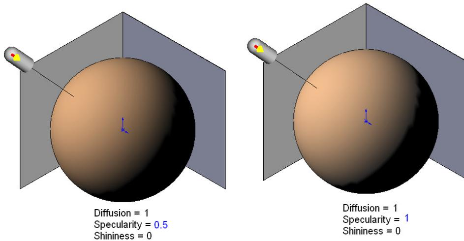
Shininess refers to the reducing speed of the specular intensity when the view is moving away from the ideal reflected ray. The lower the shininess value is, the more slowly the intensity reduces. The higher the shininess value is, the faster the intensity reduces.
