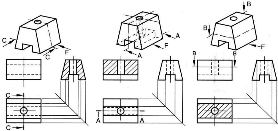
As the figure illustrates, orthographic projection facilitates the subsequent drawing of sectional views.
