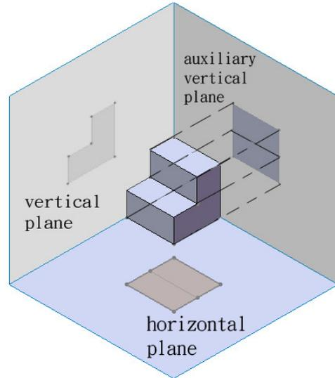
Orthographic projection of an object onto the auxiliary plane
