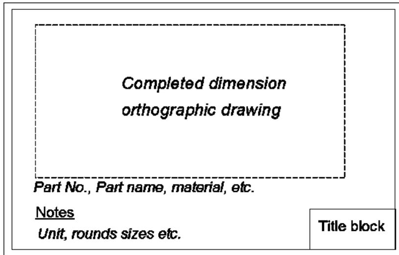
A detailed drawing can contain one drawing, or a number of separate drawings on a single sheet. It depends on the required level of details. An example of a detailed drawing is shown below:
