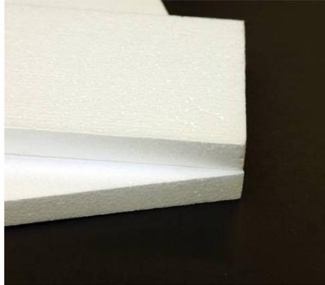
High density foam board is a material with a strong, stiff, resilient and lightweight board of polystyrene inside and covered by paper on both of its sides. There are different thicknesses and colours.
