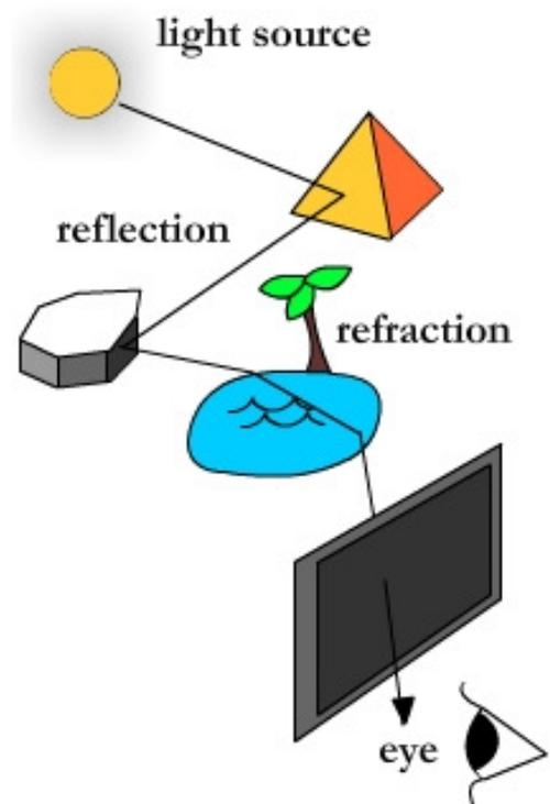
In a CAD system, the number of reflections and refractions can be decided by users. The higher the number of reflections and refractions, the better quality of image and, however, the longer the computation time will be.
