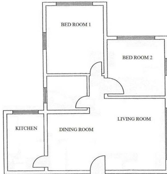
In order to indicate the features of a floor plan clearly, some conventions are used. For example, hinged doors are shown in the open position. Arcs traced by the edges of doors are also shown.
