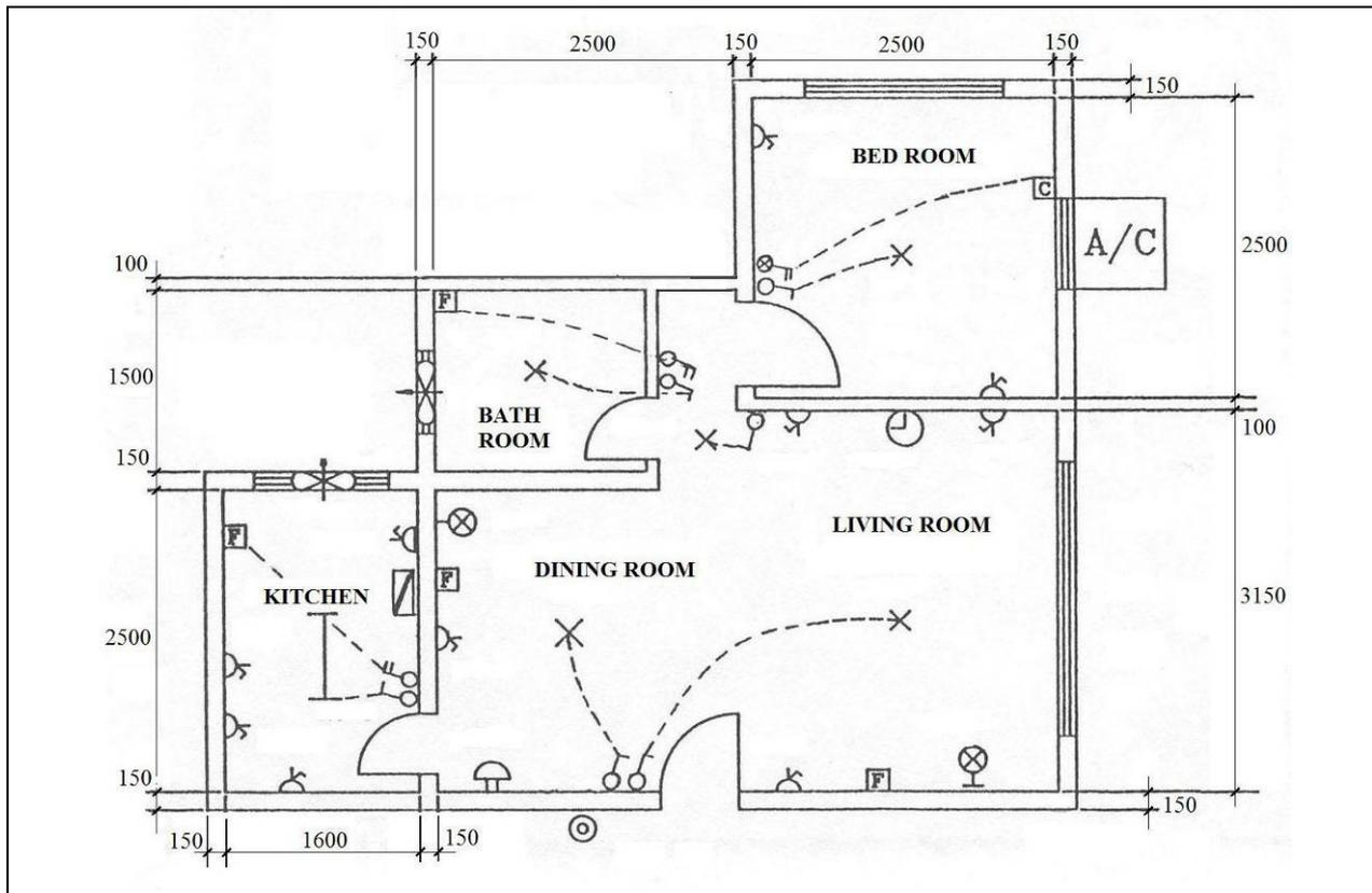
Among others, 1:100 is a scale often used in floor plans. Symbols have to be drawn in an 'appropriate size', but may or may not be on scale. An appropriate size means that a symbol has to be drawn in a size not too large to exaggerate the actual size; and not too small to create difficulty in drawing.
