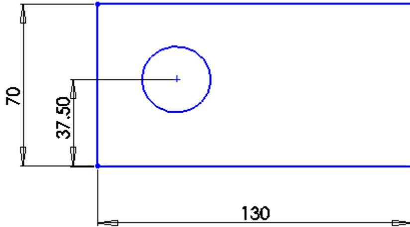
2. Extrude the profile with a depth of 45 mm;
