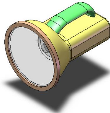
Different colours from the material colour can also be assigned to a model. For example, a designer may want to change or add a different colour to some portions of a part. This can be achieved by assigning colours to the faces or features of a part. The figure below shows a flash light assembly with assigned colours.
