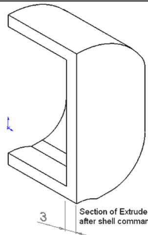
Section of Extrude A after shell command
