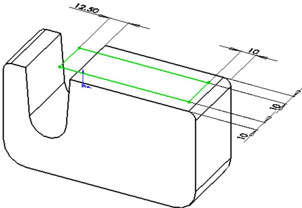
4. Use Extrude-Cut to cut downward with a depth of 45 mm.
