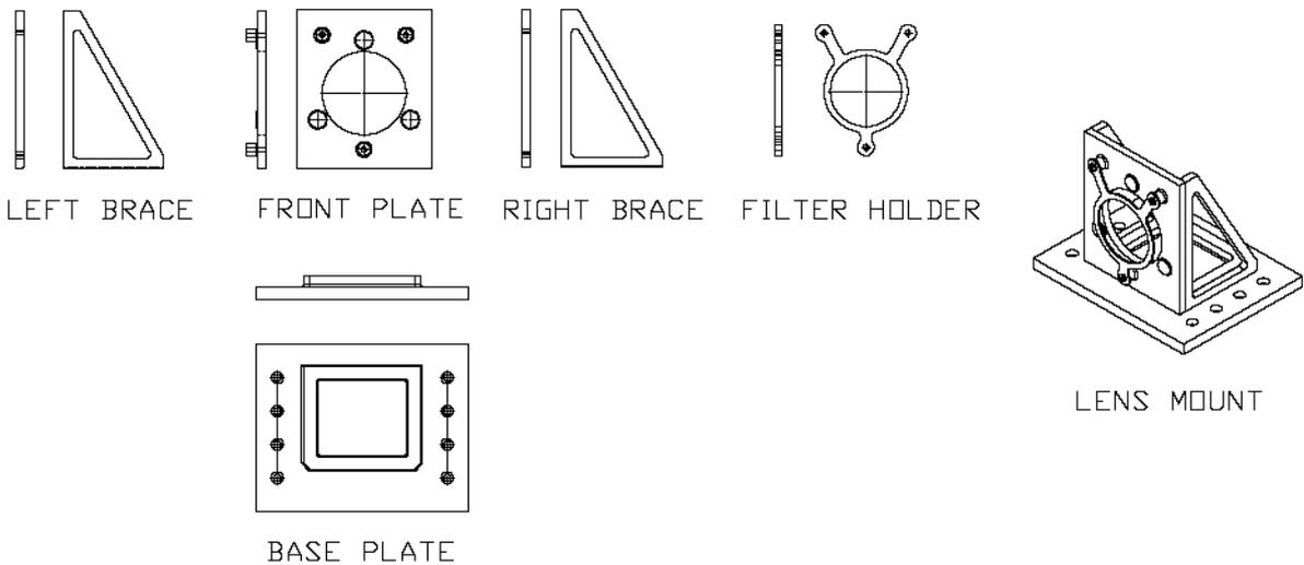
All parts and assembly drawing of a Lens Mount
