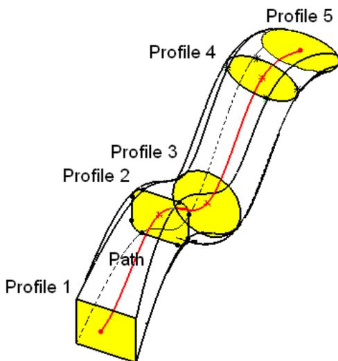
Reference plane – To create a Loft feature, two or more profiles are needed. Each profile is drawn on a reference plane. In the following example, five profiles are created on five reference planes.
