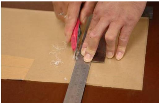
Draw the acrylic cutter along a straight edge, such as a steel rule.
