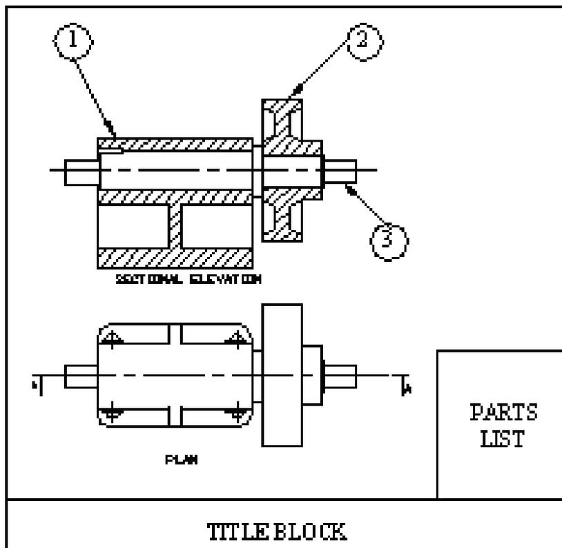
Balloon reference shows the location of parts in an assembly drawing.
