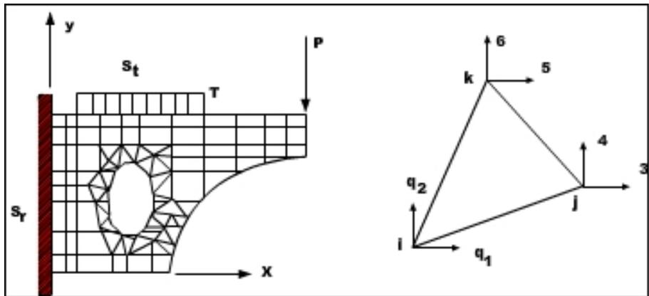
A simple FE mesh with triangular and rectangular elements for cantilever beam
