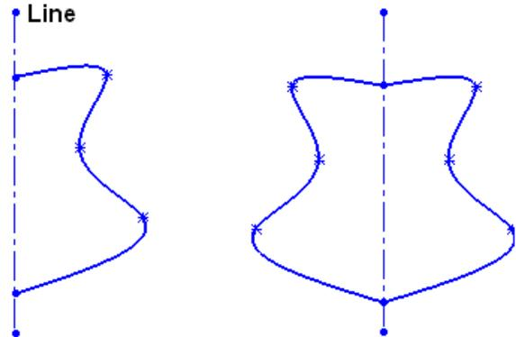
In 3D modelling, available reference geometries include axes, planes, coordinate systems, and points. For example:
